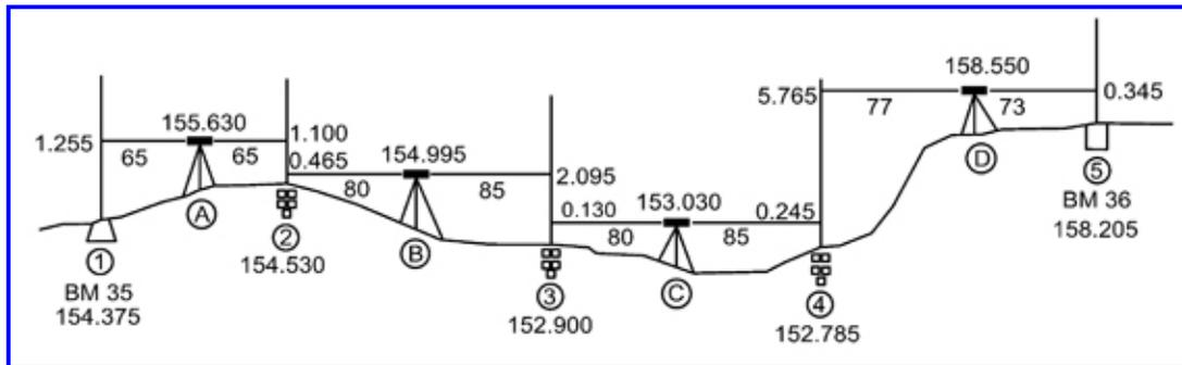
Figure 4-3. Illustration of Differential Leveling.
